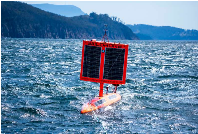
CSIRO wind- and solar-powered drone under tow to release point.
