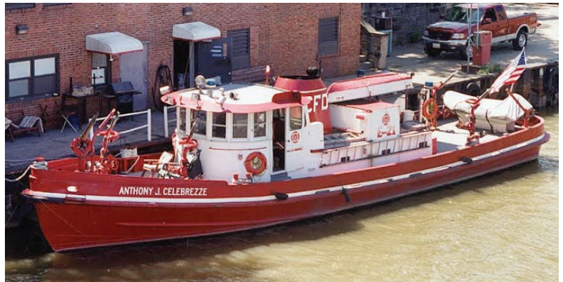
Two fire pumps aboard the Anthony J. Celebrezze can provide a total of 6,000 gallons/minute of off-ship firefighting capacity.
