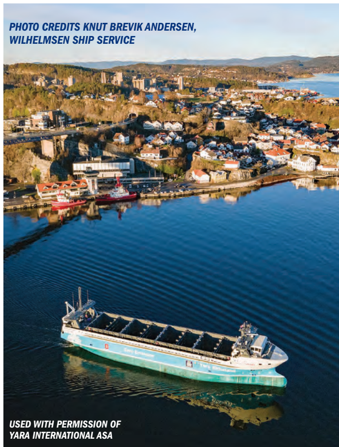
The Yara Birkeland , a 260-foot, 120 TEU electric-powered vessel operating up and down the confines of a fjord in Norway. The technology is impressive, but technical feasibility does not mean there is economic feasibility.
