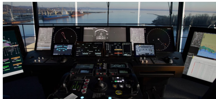
SeaQ Integrated Bridge on the cruise ship Mein Schiff Relax.
