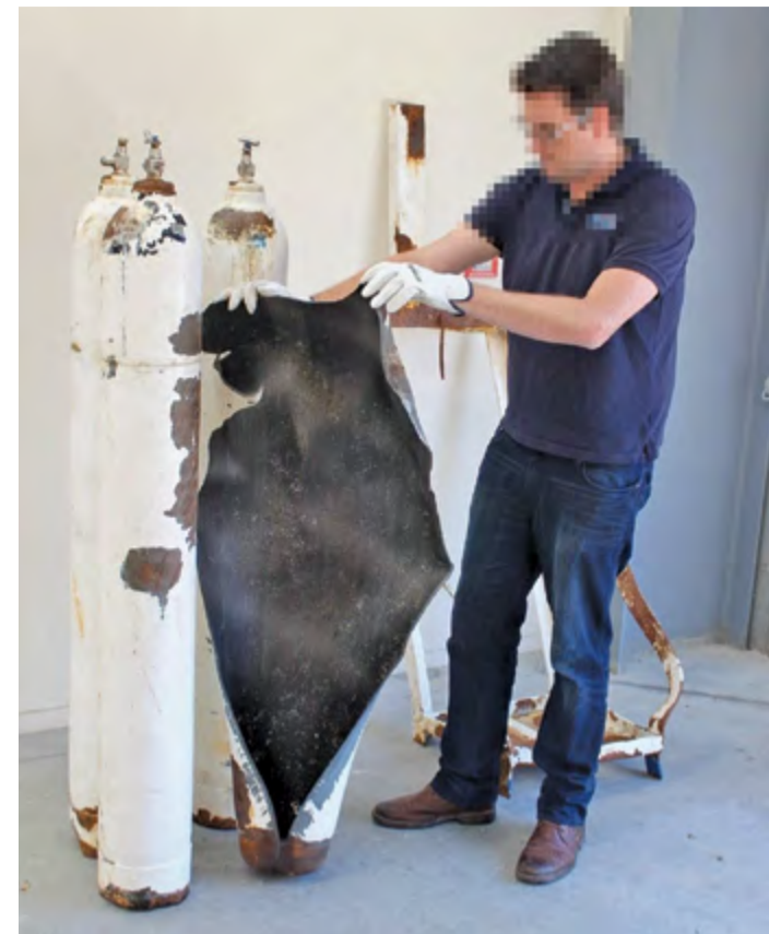
The burst high-pressure gas cylinder on Emerald Princess Picture: TAIC
